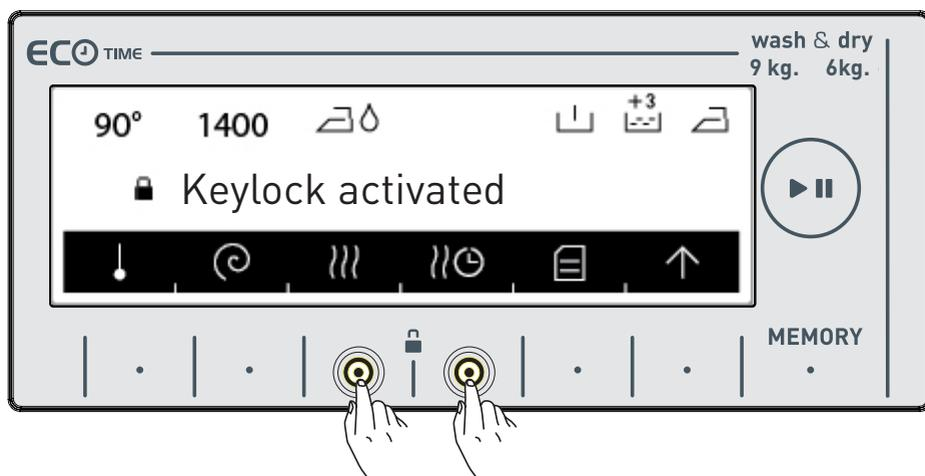
The following text will be displayed if any buttons are pressed while the child lock is engaged.
