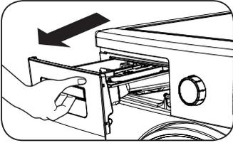
• Press the region shown below inside the detergent drawer you have pulled all the way back, and continue pulling and remove the detergent drawer from its place.
