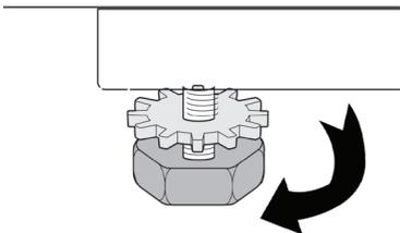
You can adjust the balance of your machine by the adjustable foot.
