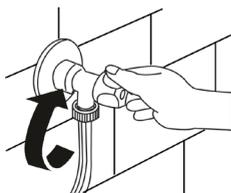
Turn off the water inlet before starting the maintenance and cleaning of your machine.
