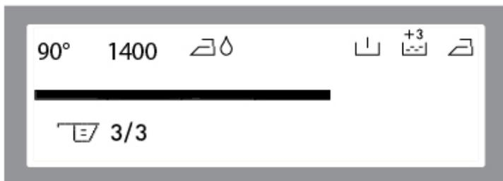
**Note:** 3/3 means a completely full detergent drawer. The amount of the detergent on the screen should be appropriate with the same amount that you put into your washing machine by detergent shovel.
